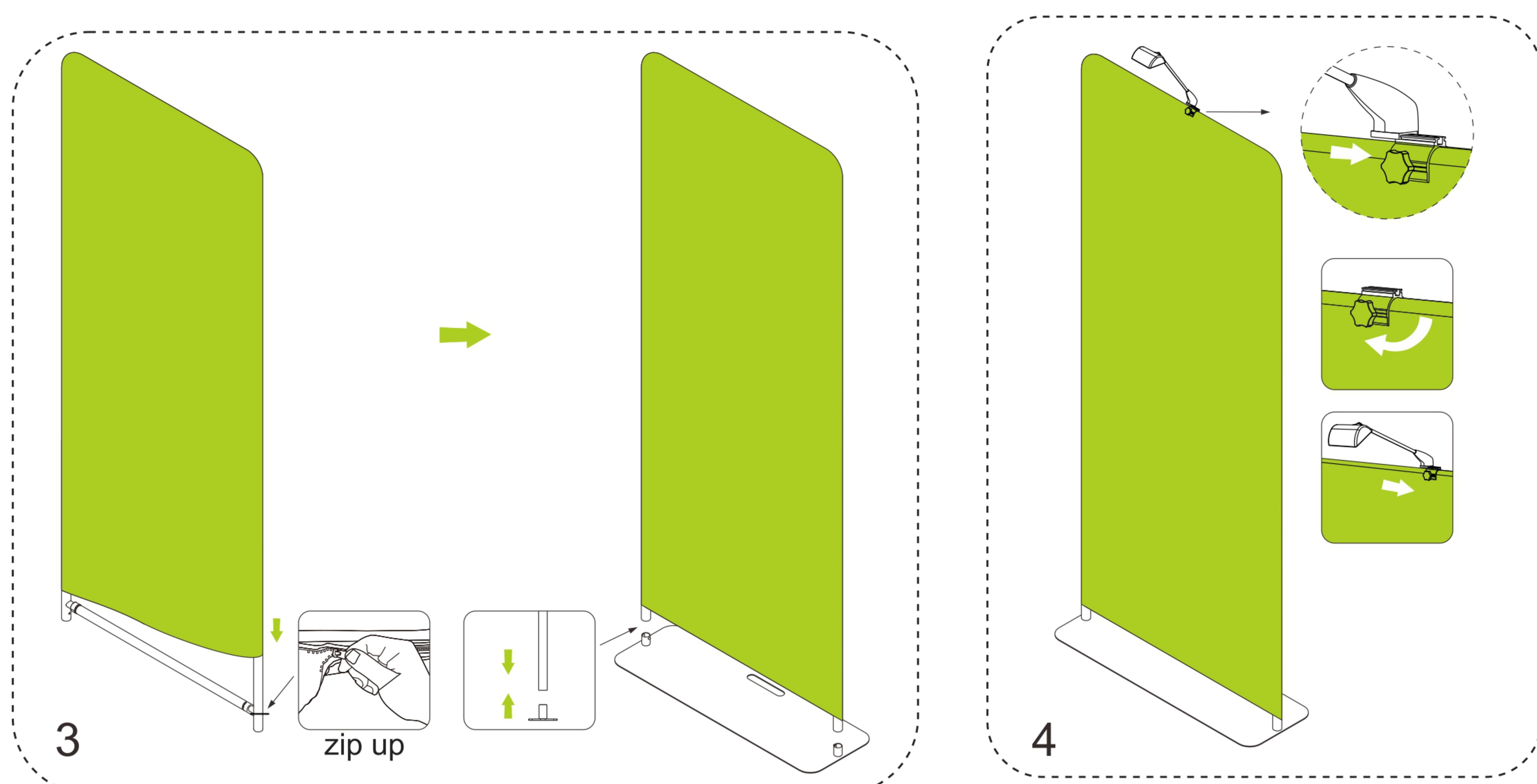
To wrap the fabric banner on the frame and zip up, afterwards install whole display stand to the base.
