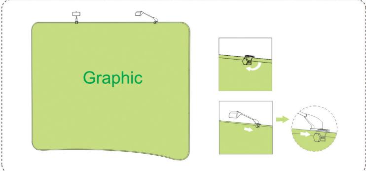
Put the light clip on the top of display and fix it with screw, then connect the light and the clip
